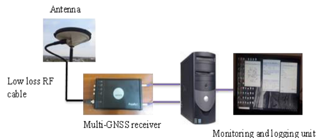
Fig. 3.1 Multi-Frequency Multi-GNSS signal receiving system
