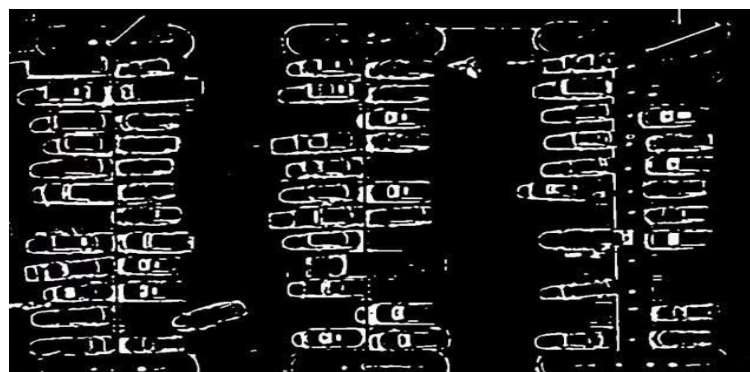
Fig 3:Image after Adaptive Thresholding
